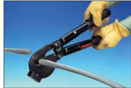
556 ACSR (aluminum conductor, steel reinforced)
